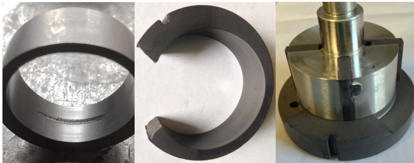
Figure 5.2 Examples of damage caused by debris in the pump: Gouged Liner (left), Cracked Liner (center), Rotor jammed by debris (right)
