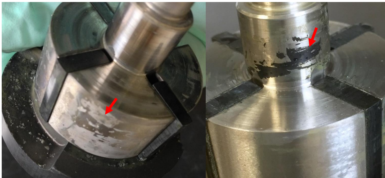
Figure 5.5 Examples of scale buildup (left) and gummy deposits (right).
