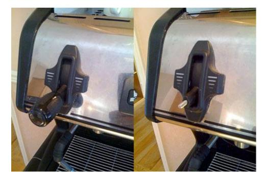
• Gently pull the front panel out from the machine and lower it down so you have access the group. It will look like the photo below:
