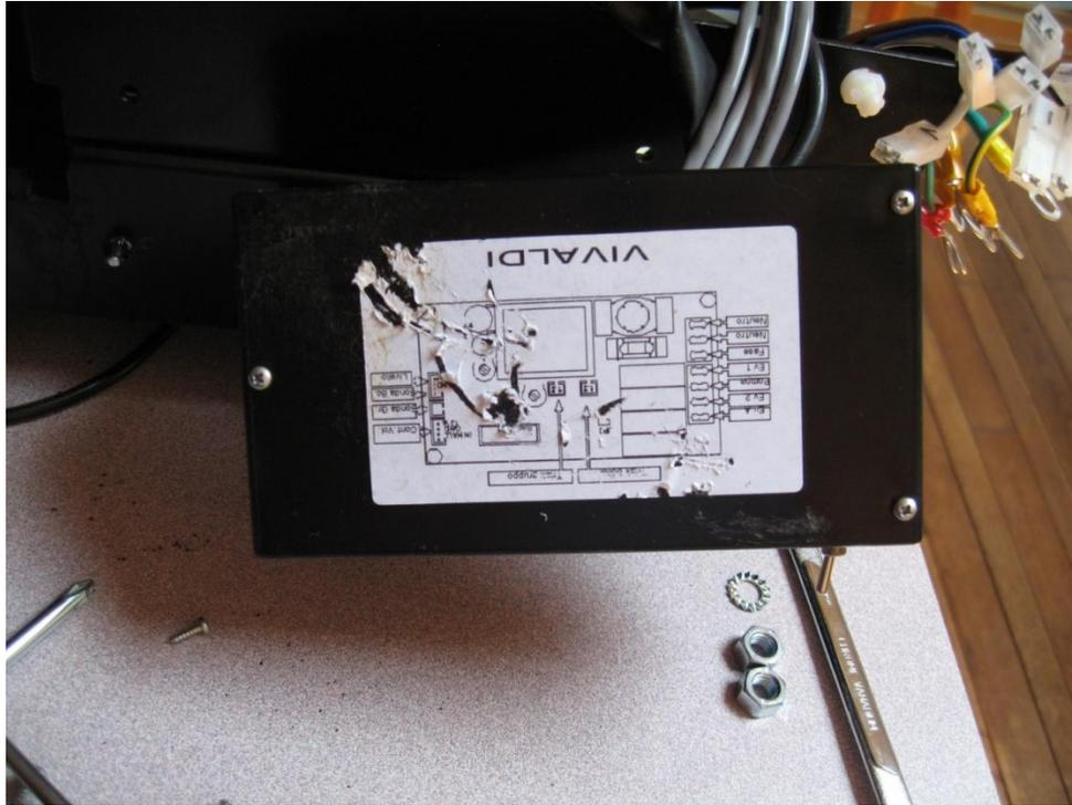
Now you can see that there are another 8 cables passing through a slot in the side of the case that need to be dealt with. Remove the three screws shown in the above photo and pull the cover off the controller box.
