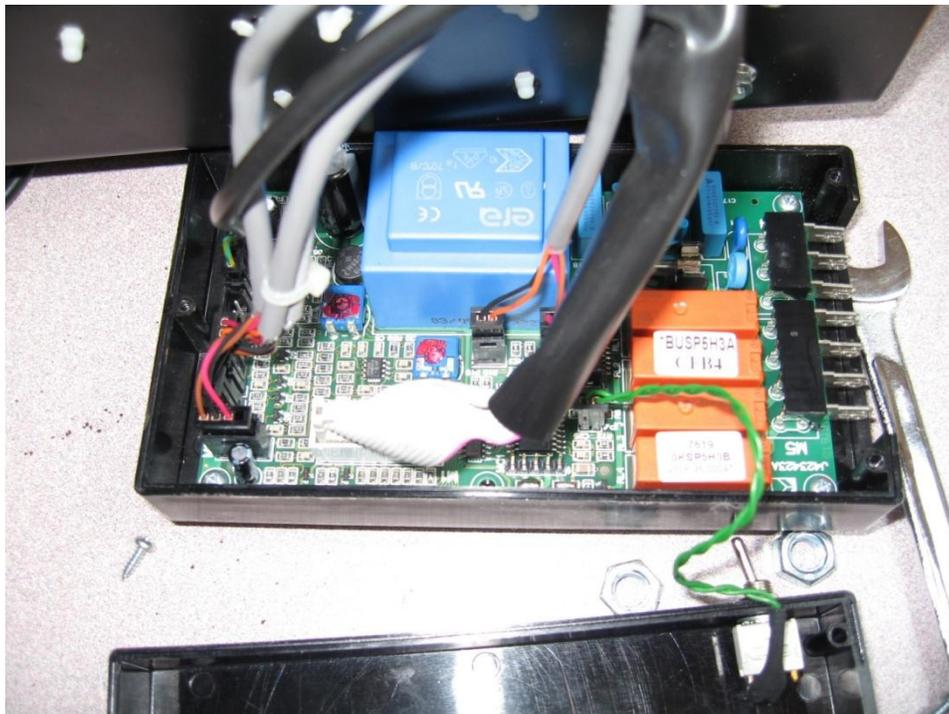
You can't see it clearly in this photo but each cable has a white silk screened label on the PC board. You should write this label's name on a piece of tape and place the labeled tape around each cable.
