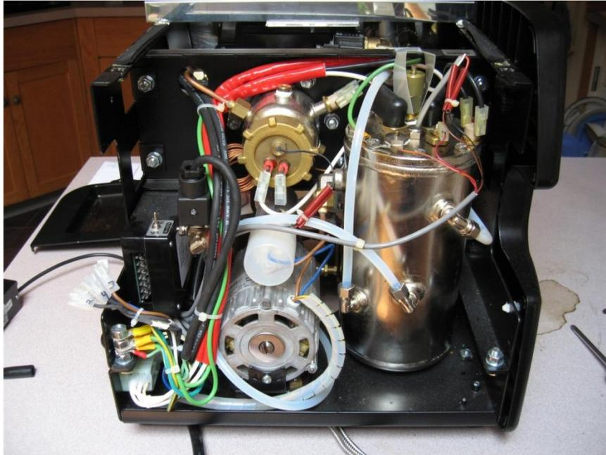
The instructions from Chris Coffee recommend removing the bolt stack and ground wires in the lower left corner. This requires a 13mm wrench. After doing this it was noted that the controller box could have been removed without this step since there was enough room to angle it up and over this bolt. Your mileage may vary depending on how your machine is built. Since these are hand built machines every one is a little different.
