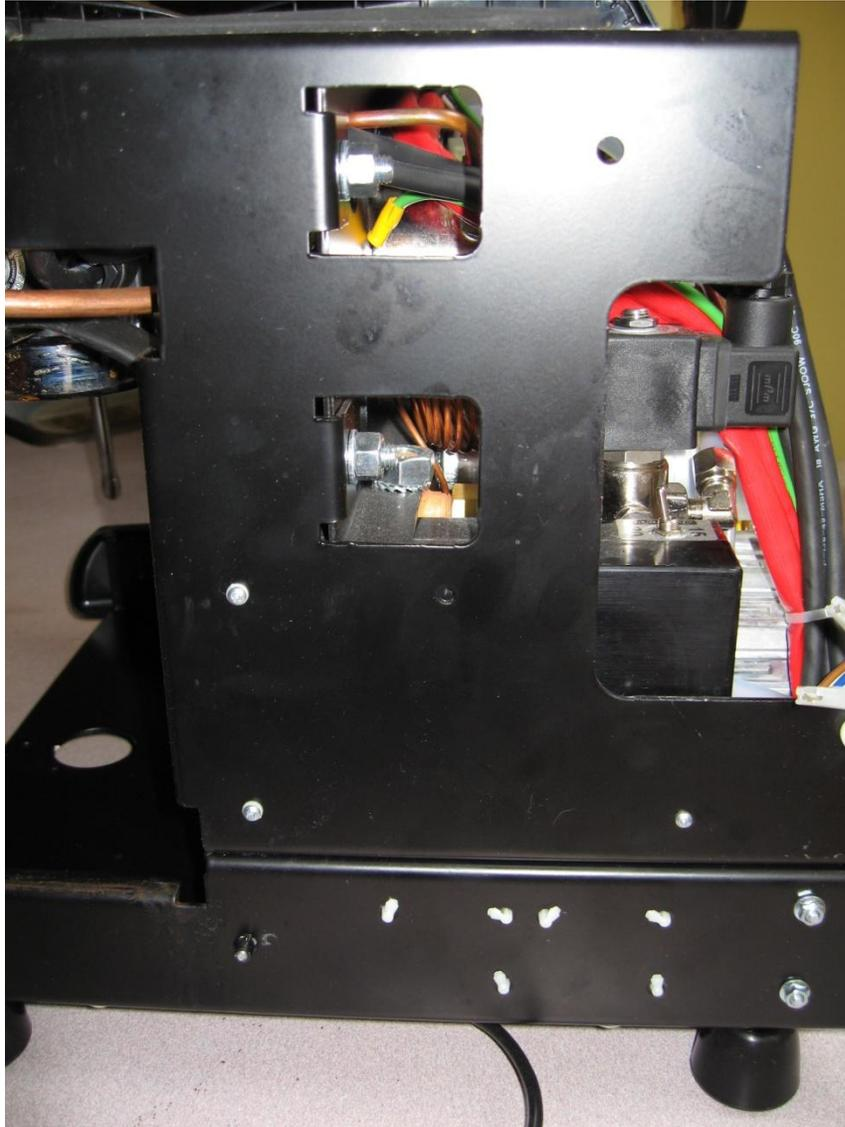
With these three screws removed, face the side panel shown above. Use your left hand to push on the controller box from the front while you angle the box up and over the ground bolt with your right hand.
