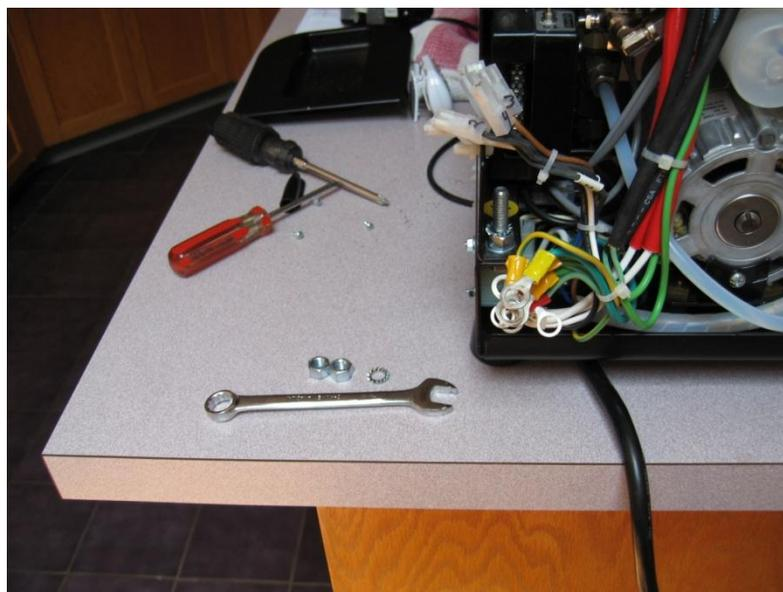
The next step requires that you unscrew the three silver Phillips screws holding the black plastic controller box to the right side of the chassis.
